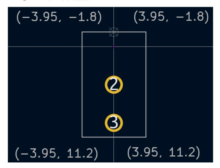
Next, switch to the F.Silkscreen layer. The silkscreen outline should be just outside of the part outline, so the silkscreen lines are moved outwards from the fabrication drawing by 0.11 mm. The exact coordinates are shown in the screenshot below, and helpful grid settings are:
