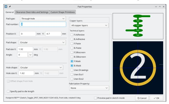
Now use the **Add a pad** tool again to place the other pad at (0, 9.4 mm). Notice that the pad number is automatically incremented and the properties including pad size and hole size are copied from the previous pad.
